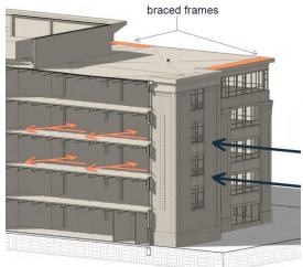
Figure 10: (above) Modified Kernick Architecture building section showing lateral load path As lateral forces are applied to the building exterior (specifically the components and cladding), bearing connections transfer the loads to the composite floor system. The load travels parallel to the original force. From there, the loads then travel perpendicularly to the braced frames at that particular level through the beams or girders. A lateral load path can be seen in Figure 10.
