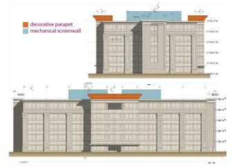
There were two types of areas on the roof that can cause snow drift. Since the mechanical penthouse stands 14' higher than the main roof, snow drift may accumulate around its walls. The penthouse is centered on the roof and is in the same rectangular shape of the MTOB footprint. Also, along the South and North facing facades, a small portion of the roof has a tall parapet as an architectural feature. See Figure 14, highlighting the areas that will cause snow
