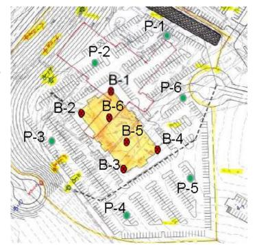
Figure 4: (above) Locations of PSI test borings. Image from PSI geotechnical report
