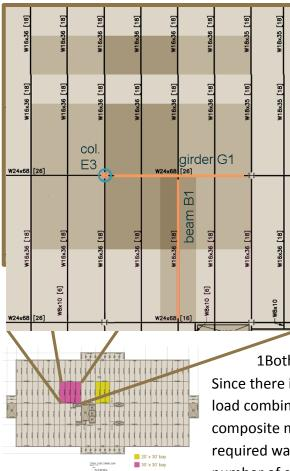
Figure 16: (above) Blown up floor plan showing the beam, girder, and column analyzed in the gravity spot check deck manual. See Figure 16 for the partial plan and appendix B for hand calculations.
