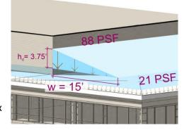
Figure 15: (above) Drift load sketch
