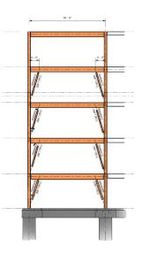
Figure 8: (above) Modified AES braced frame elevation
